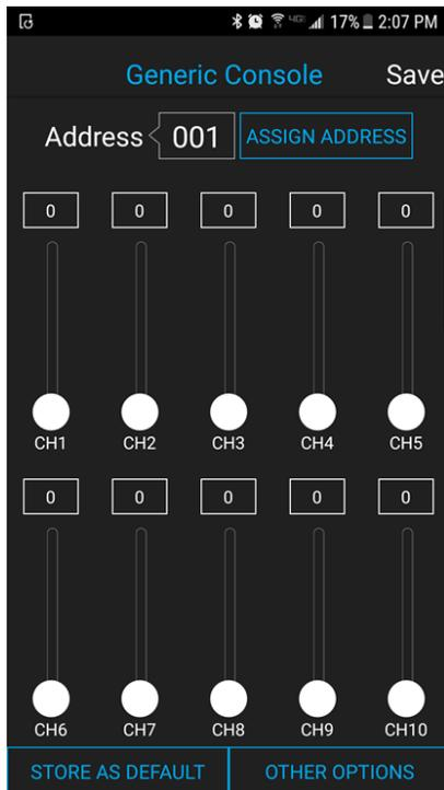
To set the DMX address, first connect the Precision Z DMX to the DMX Programmer app by Gantom as was outlined earlier in this document. With the Generic Console control screen open, you should have full control of the fixture using the CH1 slider. If the light fixture is connected to the app but is not responding, try power cycling the light fixture.
