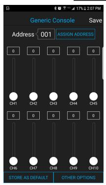
To set the DMX address, first connect the Gantom Juni DMX to the DMX Programmer app by Gantom as was outlined earlier in this document. With the Generic Console control screen open, you should have full control of the fixture using the CH1 slider. If the light fixture is connected to the app but is not responding, try power cycling the light fixture.
