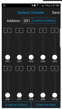
To set the DMX address, first connect the Precision Z DMX to the DMX Programmer app by Gantom as was outlined earlier in this document. With the Generic Console control screen open, you should have full control of the fixture using the CH1 slider. If the light fixture is connected to the app but is not responding, try power cycling the light fixture.
